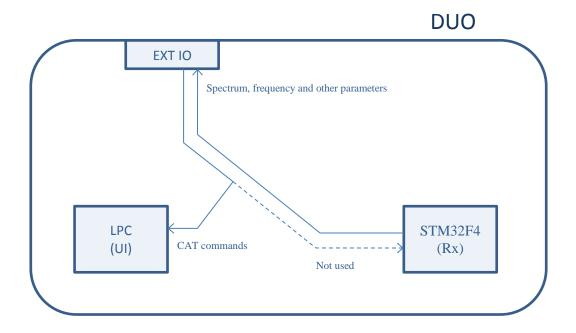
The data sent by the STM32F4 are divided into two groups: the spectrum and the parameters (frequency, states and various settings). The parameters are sent every 250ms and the spectrum is sent every 150ms.
